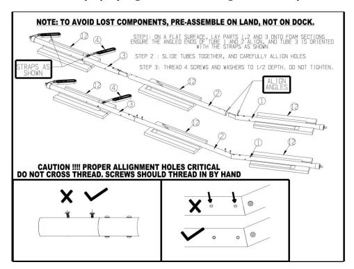
Step 2 – Slide tubes together, aligning threaded holes in the aluminum brackets with the tube screw holes. Install 4 screws by hand. Do not cross-thread. Screws should insert easily. Tighten only halfway to allow for easier alignment of screws on the opposite side.
