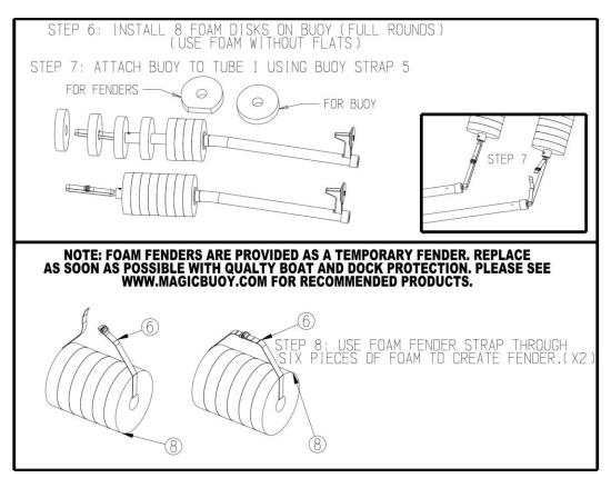
Step 8 – Assemble temporary fenders using packing foam (see diagram).
