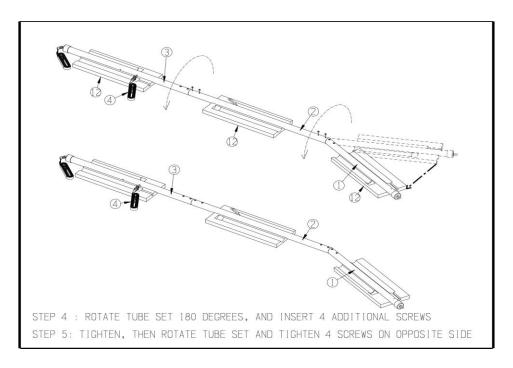
Step 5 – Rotate back 180° and finish tightening the original 4 screws.
