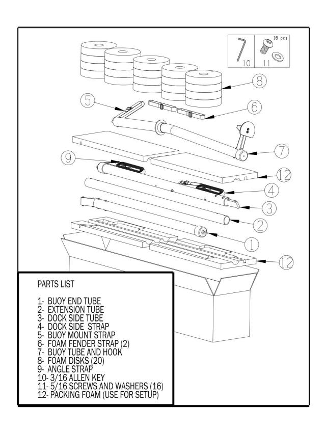
Important: Assemble the main tube set on land. These components do not float.
